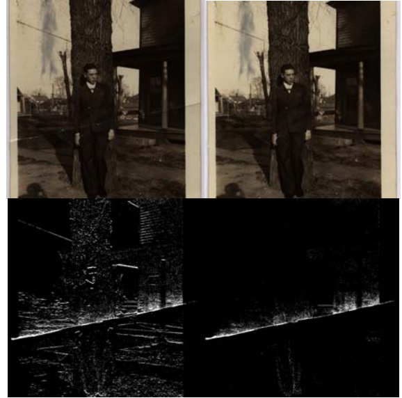
Figure 6: UL: Scanned image. UR: Repaired image. LL: Absolute value of the y derivative before the alignment step. LR: After alignment.
