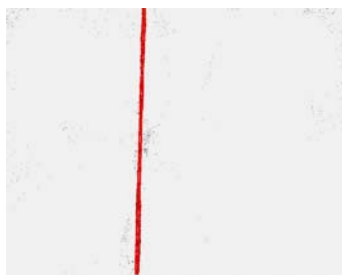
Figure 10: The trimap for Fig. 8a: red pixels are defect, light grey are non-defect and black are unknown (appear sparse and small in this case).
