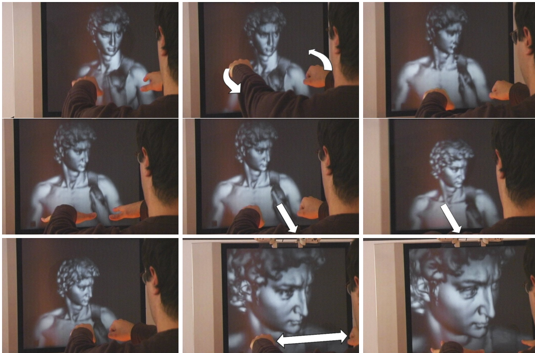
Fig. 6. Successive moments of interactive manipulation of the David 1mm dataset (56M triangles) using our 7.4Mbeams display coupled with the vision based hand tracker and driven by a single PC.
