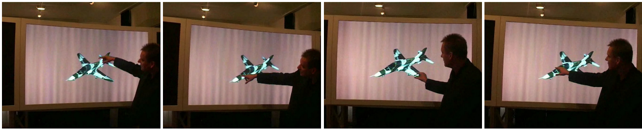
Figure 3: Holographic display example. Images that were taken from different positions in front of the display. Objects appear at fixed physical positions.
