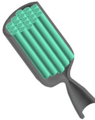
Figure 4: Perspective view of the assembled Catiuscia engine. All modules discharge in the same nozzle.
