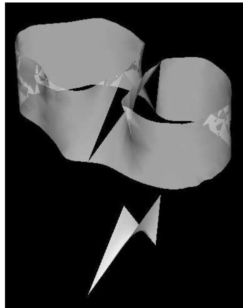
Fig. 10. Generation of three patch-shells for bifurcation. The three B-Spline patches resulting from the automatic shape reconstruction algorithm.
