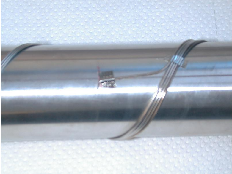
Figure 9: Photo of the pin internal part with the spiral and the thermocouple wires.
