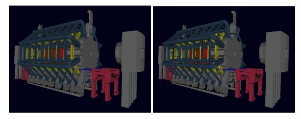
Figure 1: A view of the whole ATLAS Experiment Pit. Comparison between full (left, 1,072,858 triangles) and adaptive resolution (right, 41,487 triangles).
