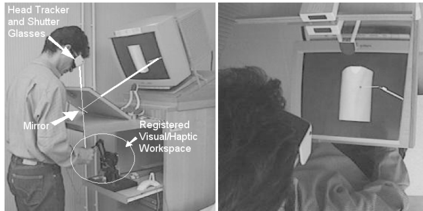
Fig. 1. Haptic Workbench Configuration. The user looks into a mirror through shutter glasses and perceives the virtual image within the workspace of a PHANToM haptic device which controls needle insertion. The user can thus manipulate and feel the needle with his hands without obscuring the display.
