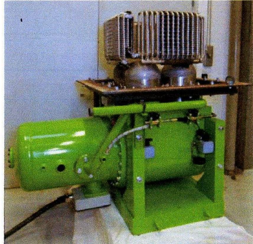
*The newly developed 35 kW<sub>e</sub> Stirling engine for biomass combustion plants (Source: BIOS Bioenergy Systems, Austria & Henrik Carlsen, Denmark, 2003)*
