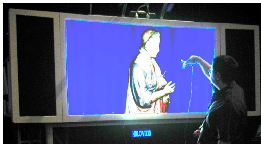
Fig. 6. Massive model visualization on a 50Mpixel spatial 3D display. The display has a screen dimension of 1.6x0.9 meters, and provides continuous horizontal parallax. Interactive rates in the manipulation of massive geometric models are guaranteed by a cluster-parallel spatial 3D display aware coarse grained multiresolution technique.
