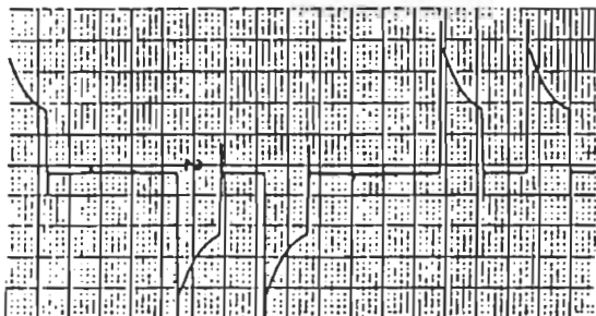
ac line current; 0.5 A/div, 1 ms/div
