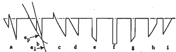
Fig. 8: Typical waveforms of the 8 thyristor converter for E_d=0.17
