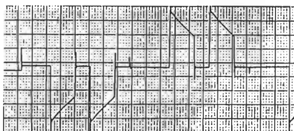
ac line current; 0.5 A/div, 1 ms/div
