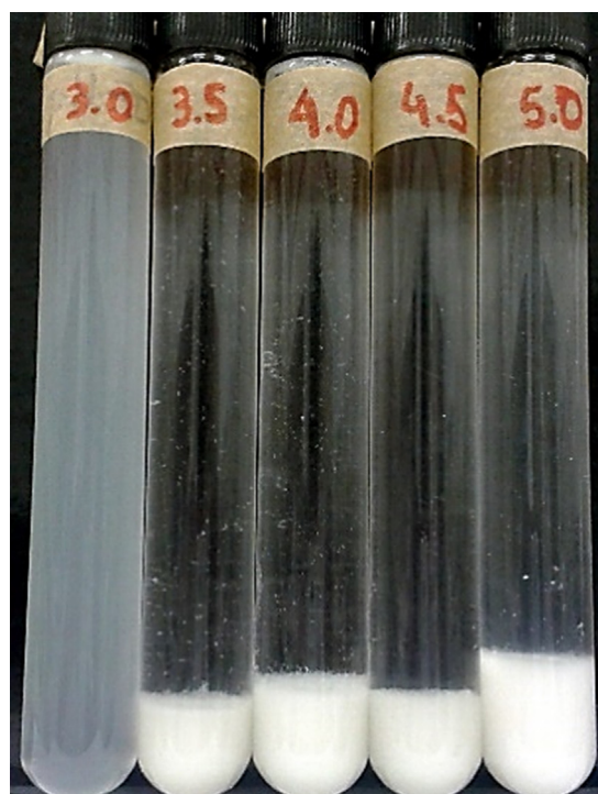
Fig. 2. Evaluation of process yield by the sedimentation efficiency of the coacervates produced with different pH values (3.0, 3.5, 4.0, 4.5, 5.0).
