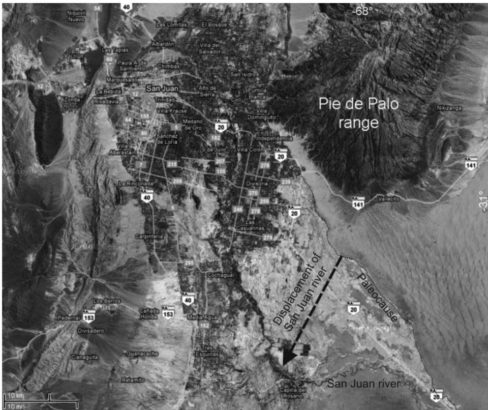
Figure 4. Satellite image obtained, where the migration of the San Juan river course is observed over a period of time.
