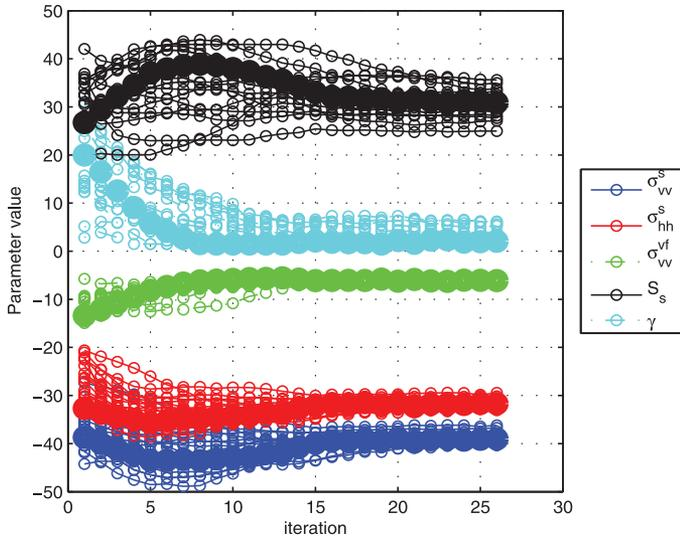
Fig. 3. Parameter values (dB) versus iteration using random initialization of the end-member parameters showing rate of convergence and stability when converged. It also shows compensation between correlated parameters.
