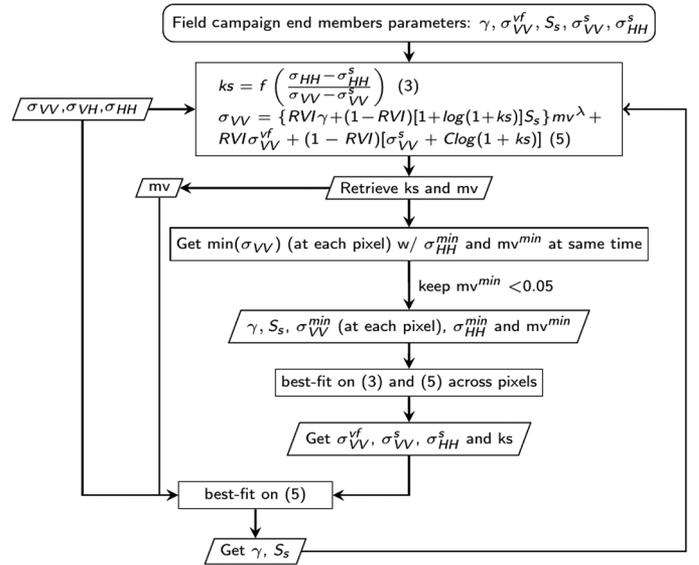
Fig. 2. Conceptual flow diagram of the iterative process parameter estimation (*Intercept* and *Sensitivity*). Note that no use of ancillary data is required.
