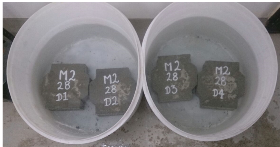
Figure 6. Paving stones made from M2 concrete mix using recycled aggregates.
