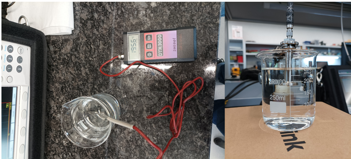
Figure 1.7: Water measurement with probe DAK 3.5 manufactured by Speag . The water is near to 20^{\circ}\text{C}
