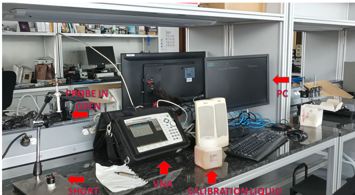
Figure 1.4: Set measurement system calibration (VNA - Probe) open circuit (Open)
