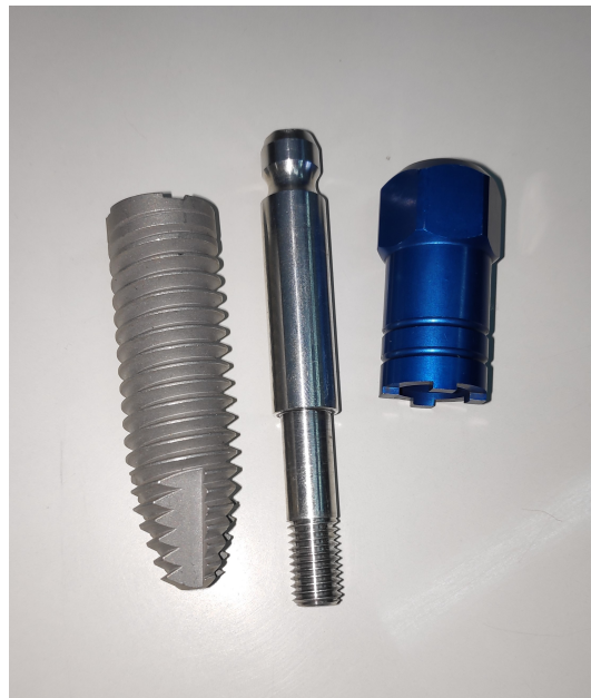
Figure 3.6: Photo of the real implant in enlarged scale (5:1).
