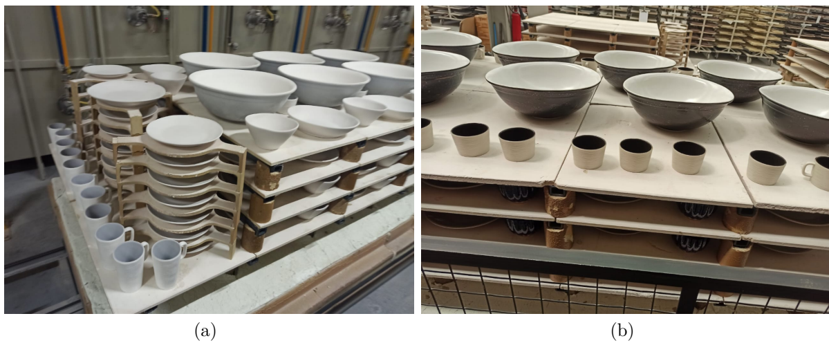
Figure 1.2: a) Before and b) after being fired in the oven.
