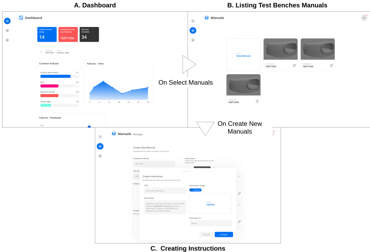
Figure 5.3: Screens of the admin application prototype. A. The main dashboard, B. Listing test bench manuals, and C. Form used to create the manuals' instruction.
