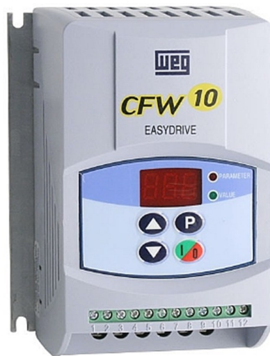
Figure 3.10: Picture of the motor driver WEG CFW10
