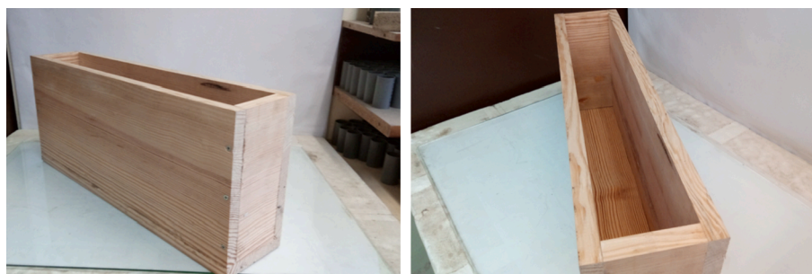
Fig. 5. Lightweight blocks mold (60 cm × 25 cm × 10 cm).
