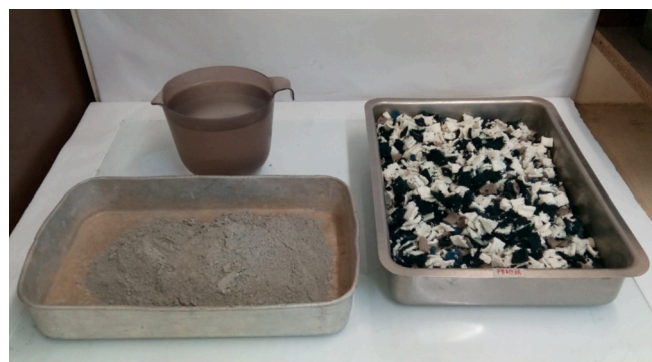
Fig. 3. Materials used in the mixture's composition: TW, water, and Portland cement.
