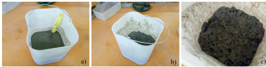
Fig. 4. Preparation of the mixtures: a) Cement and water mixture; b) TW incorporation; c) Final mixture.
