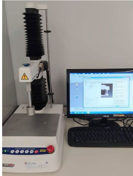
Figure 19. Texturometer with 30 Kg load cell and P/35 aluminium cylindrical probe.
