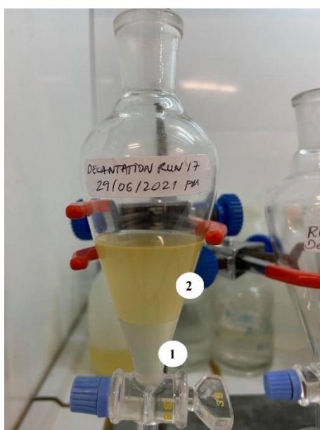
Figure 20 - Phase separation using a decanting funnel. 1- heavy phase; 2-light phase.
