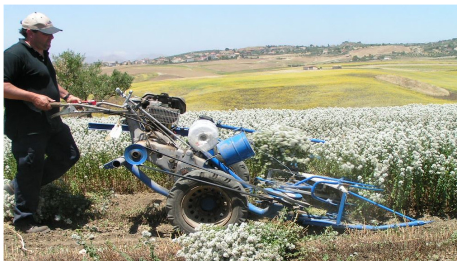
Figure 1. Modified BCS 622 reaper-binder used during the mechanical harvesting test.
