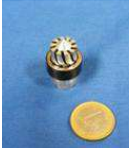
Figure 3.16 – Detail of microturbine fluid dynamic part
