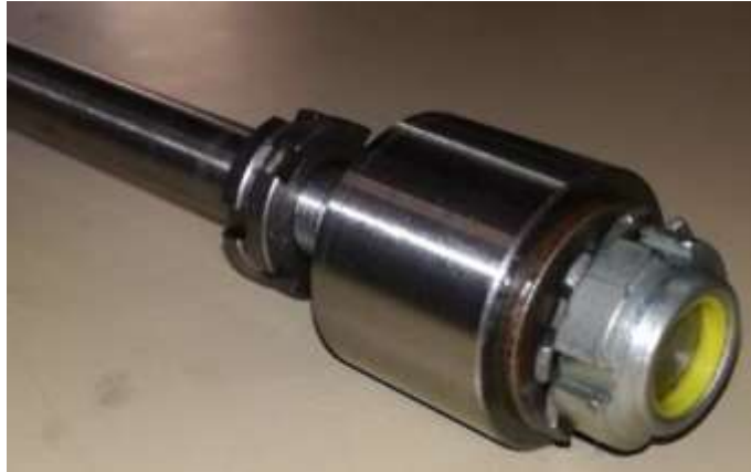
Figure 2.3 – Prototype of the custom shaft with interchangeable journals
