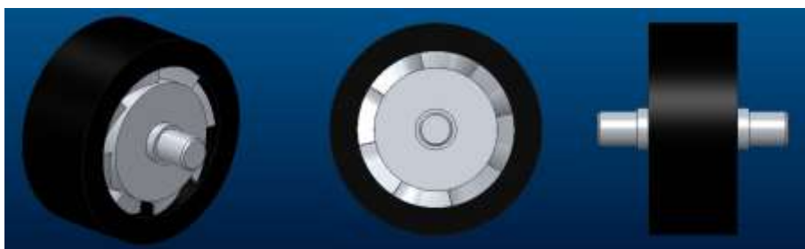
Figure 3.21 – 3D CAD of real rotor assembly to be simulated
