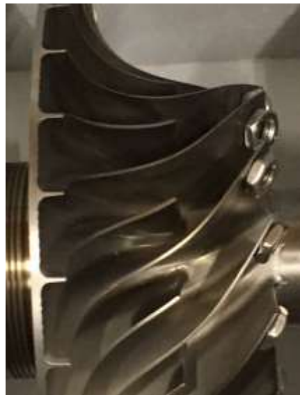
Figure 5.9: compressor impeller: detail of main and splitter blades (additional masses on some blades are present for dynamic structural mistuning purpose in impact test)
