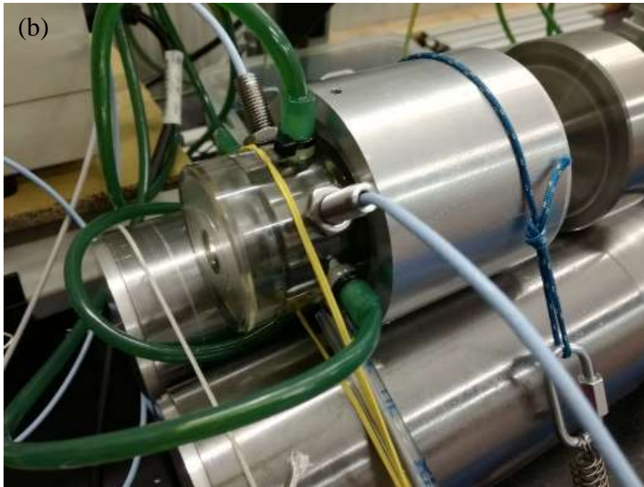
Figure 2.29 – Proximity probes arrangement: (a) in previous setups, (b) in the new RK final setup
