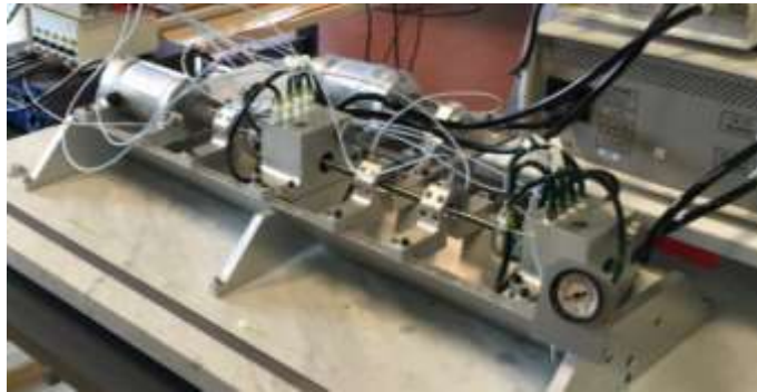
Figure 2.6 – Rotor assembly mounted with custom shaft in configuration 2
