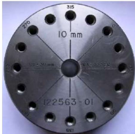
Figure 3.10 – Fly-wheel mass with holes for balancing masses
