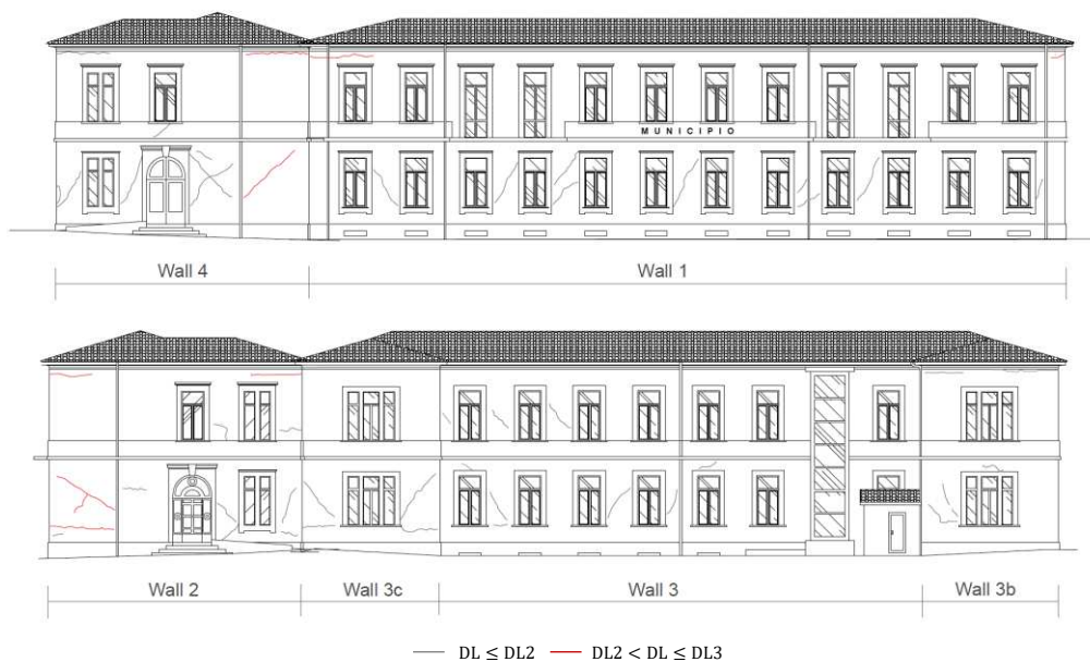
148 Fig. 2 Damage survey detected on the Pizzoli's town hall during the in-situ inspections after the mainshock of 149 18/01/2017— figure adapted from Degli Abbatini et al., 2021a.
