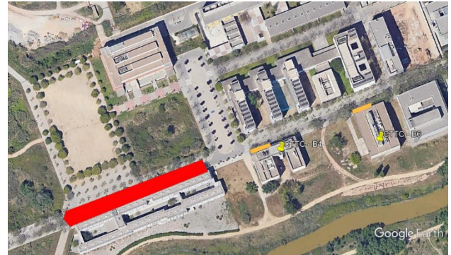
Figure 4. Parc Mediterrani de la Tecnologia where CTTC buildings are located. In red, area with strong multipath conditions. In orange, indoor/outdoor transition areas.
