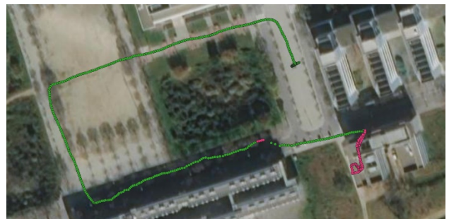
Figure 9. Estimated “CTTC-LAB” trajectory. Green dots indicate positions provided by the GNSS while red dots are the ones provided by camera-based tracking system.
