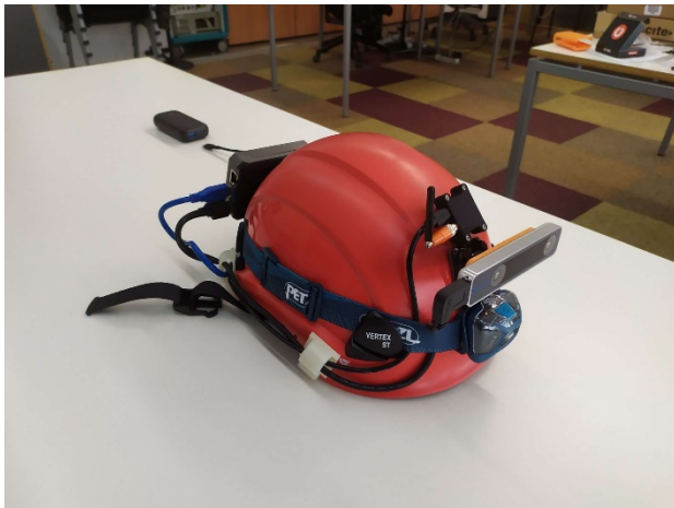
Figure 2. IOPES positioning system mounted on a Helmet.
