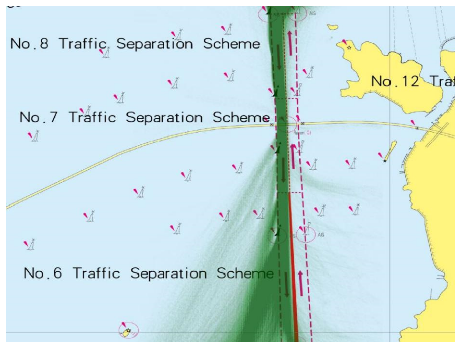
Figure 8. Traffic separation scheme (TSS) in the main navigable span of the Jintang Bridge. The AIS data are also displayed by black points.
