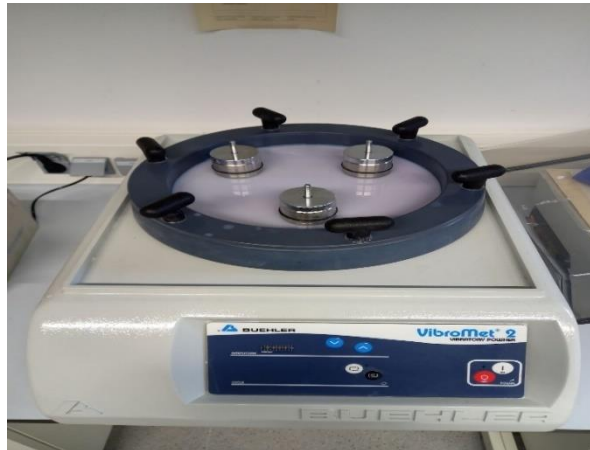
Figure 46: Buehler Vibromet 2 vibratory polisher.
