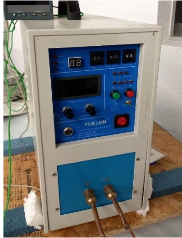
Figure 36: YUELON model HF15-A inductor.
