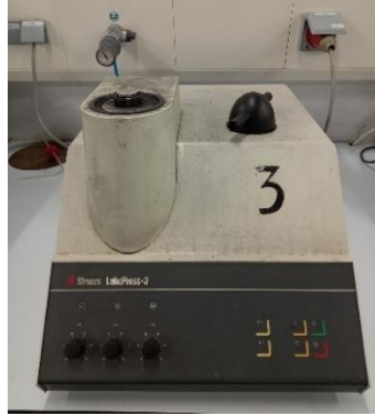
Figure 44: Struers LaboPress-3 hot coating machine.
