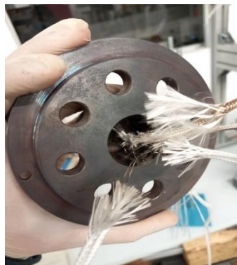
Figure 49: Four 4 thermocouples welded inside the nozzle.
