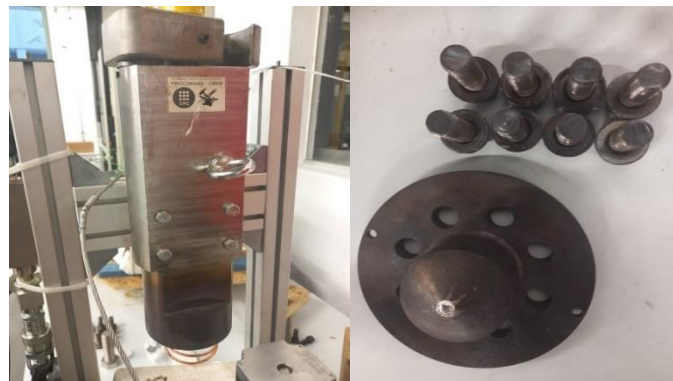
Figure 28: The extruder body, the nozzle, and the 8 bolts.
