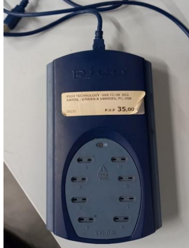
Figure 40: TC-08 thermocouple data logger.
