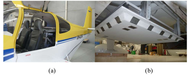
Fig. 1: (a) Microwave interferometric reflectometer (MIR) instrument and up-looking array mounted inside the airplane, and (b) down-looking array covered with a radome hanging from the airplane's fuselage [1]
