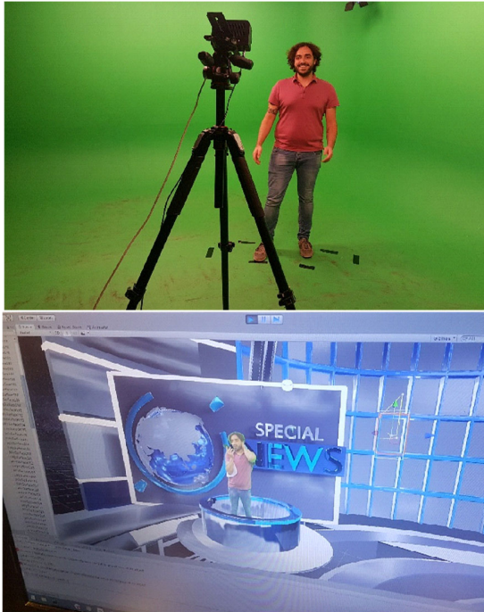
Fig. 11. Live capture of the presenter and its integration in the virtual scenario.
