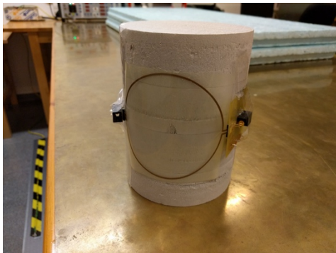
Fig. 2. Developed double-loop curved probe employed to measure simultaneous the E-Field and the H-Field
