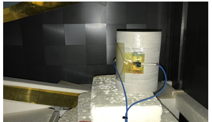
Fig. 10. The curved probe placed within the EUROTEM@2 cell
