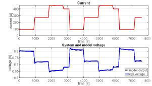
b)Top: cell current. Bottom: cell output voltage and model approximation.
