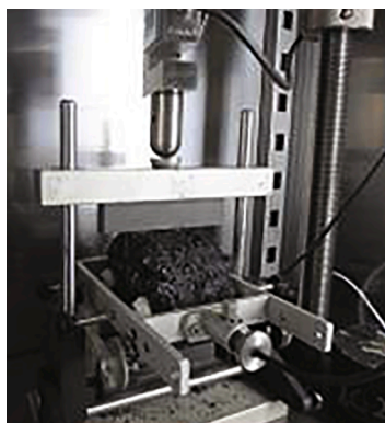
Fig. 4. Stiffness test equipment.
