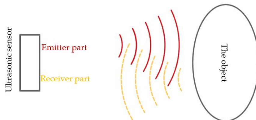
Figure 2. The principle behind distance measurement with sonar sensors.
