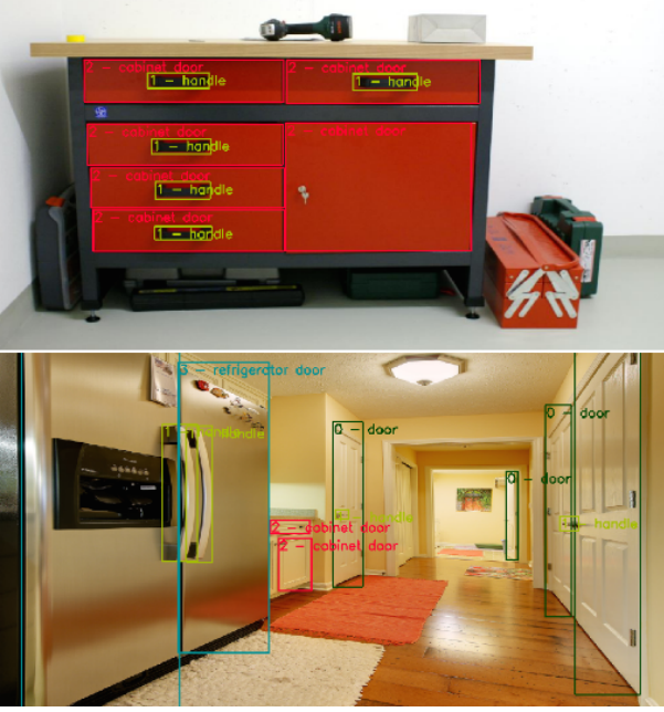
Fig. 2 Examples of annotated images from the training dataset used for building the door and handle detection model. The bounding boxes enclose the objects, with the corresponding label, that should be identified by the model.
