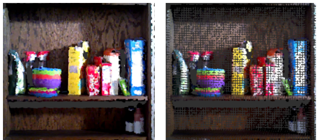
Fig. 4 On the left, the raw point cloud. On the right, the downsampled point cloud using a voxelized grid approach.
