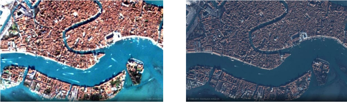
Figure 1: Sentinel-2(ESA) image with a 10m resolution (medium resolution) (left) vs. satellite Pléiades (Airbus) image with a 50cm resolution (high resolution) (right) [61]
