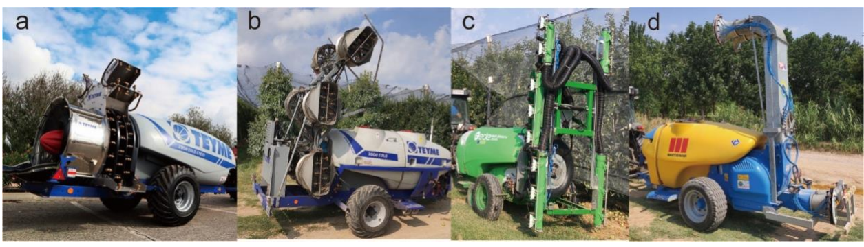
130 Fig. 1. The sprayers used for the field trials: a) Teyme EOLO 2000 conventional axial-fan sprayer b) Teyme prototype 131 sprayer equipped with six independent electric axial fans; c) Fede orchard sprayer equipped with vertical booms 132 (VERTICAL); d) Martignani pneumatic sprayer.
