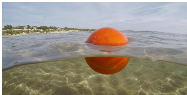
Fig. 1. Lagrangian Drifter deployed at coastal area, in the Mediterranean Sea, within the tests of the EC-founded MELOA project [3].
