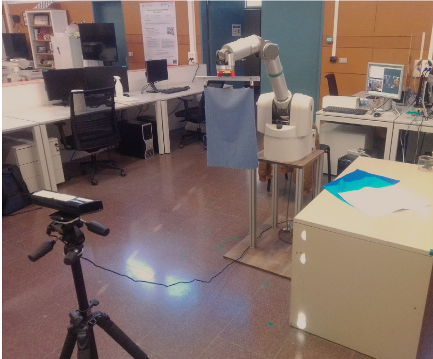
Fig. 3. Experimental setup for the recording of real world data. On the left, the depth camera. On the right, the robotic arm with an affixed hanger.
