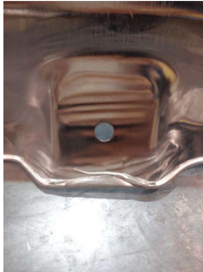
Figure 10. Overlapping through hemming
