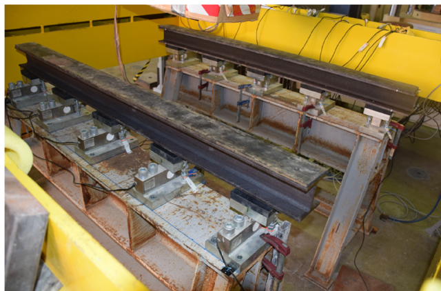
FIGURE 7 Support system for the tested specimens
