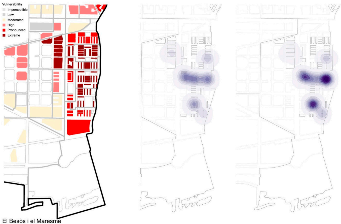
Figure 12. Comparison of maps of results obtained in the study of detection of areas of vulnerability (on the left) [24] and the present study (density of buildings in the center, and density of dwellings on the right) in the El Besòs i el Maresme neighborhood.
