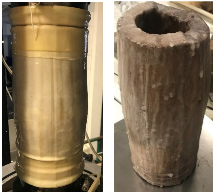
Figure 7. Soil sample at the end of the test (left) and after being coated with paraffin (right).
