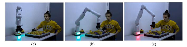
**Fig. 5.** Collaboration types. (a) Non-physical collaboration: the robot is selecting the compartment to place a token and the human monitors how the robot does its part of the plan. (b) Indirectly physical collaboration: the human and the robot move to place a token in different compartments without exchanging forces. (c) Directly physical collaboration: the human moves the robot exchanging forces while the robot remains in admittance mode.
