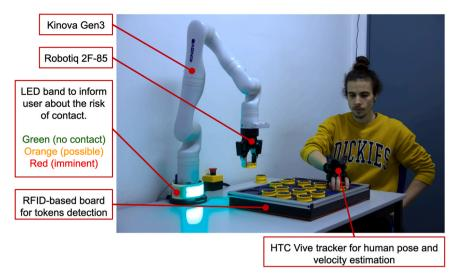
Fig. 2. Setup of collaboratively filling a tray: example of an industrial kitting task used during the validation of this work.
