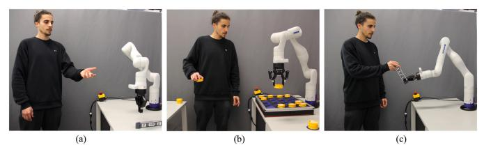
**Fig. 1.** Examples of collaborative tasks in which the human and the robot continuously share both the workspace and the execution of the task. (a) Example of a collaboration in which the human is stopped asking the robot for a tool. (b) Example of a kitting task in which the human and the robot collaboratively fill a tray with tokens. This task was used during the validation. (c) Example of a collaborative hand-over of a tool in which the robot and the human exchange forces.
