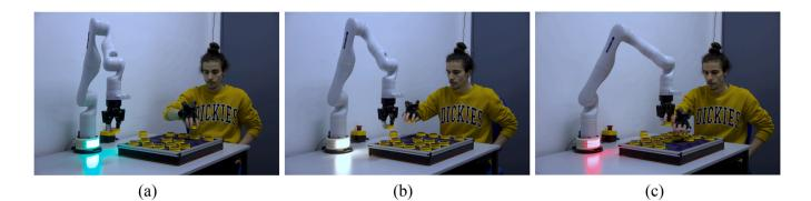
Fig. 6. Collaboration risks. (a) Low risk - green light: there is not any potential detected collision. (b) Medium risk - orange light: the robot has detected a possible collision. (c) High risk - red light: the detected collision is imminent.
