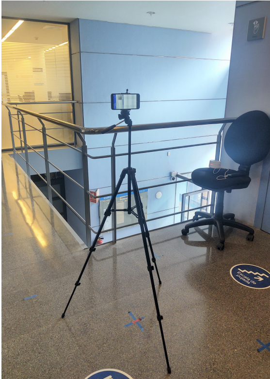
Fig. 2. Data collection in the proximity of AP2 and with the STA in vertical and landscape orientation (VL). The reference points are labelled with blue tape on the floor.
