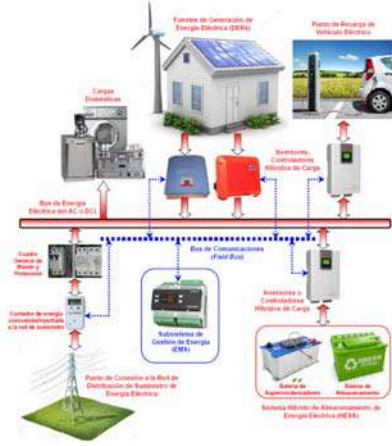
Fig. 1. Conceptual block diagram of the structure of a domestic microgrid around a domestic prosumer
