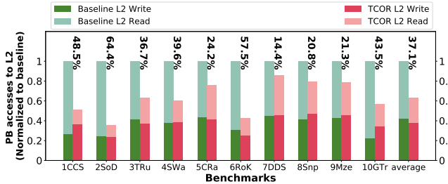
Figure 15: Parameter Buffer accesses to L2, normalized to the baseline (128KiB Tile Cache).
