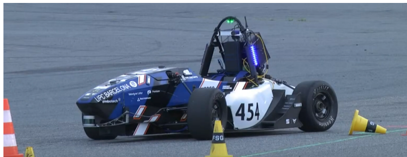
Figure 2.1: A naïve team's out-of-track autonomous car thinking GNSS as an initial solution would "kind of work", Formula Student Germany 2021.
