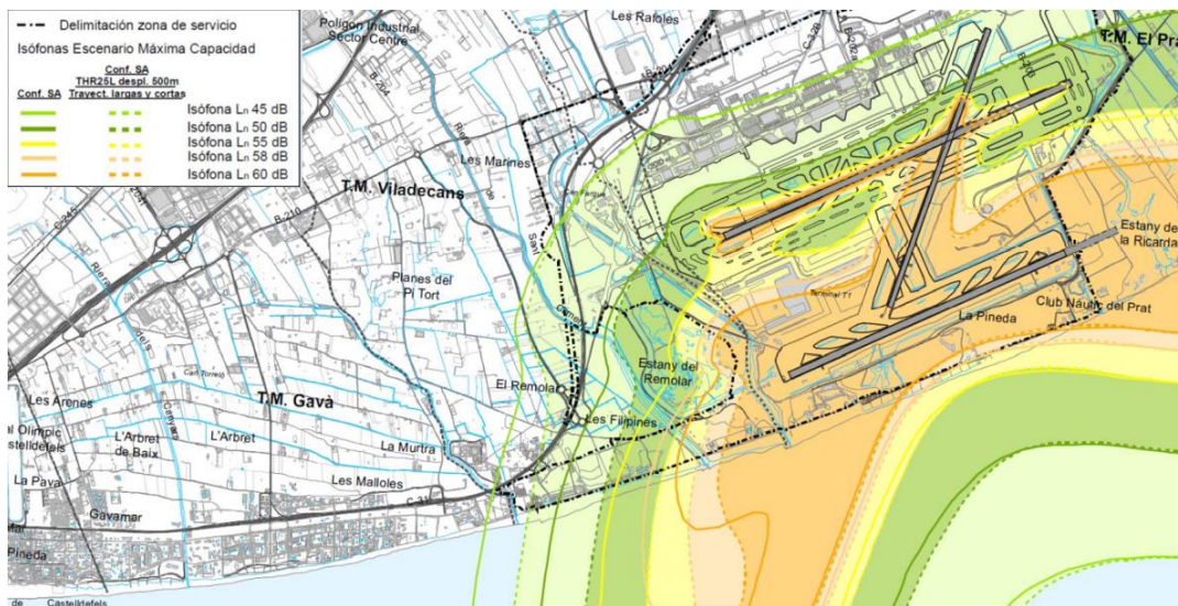
Figure 52: Acoustic isophones of the night-time operations in the BCN airport (Source: AENA)
