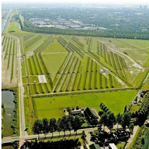
Figure 22: The shape of the fields next to the Schiphol airport help reduce the noise in the surrounding areas considerably (Source: Schiphol airport)
