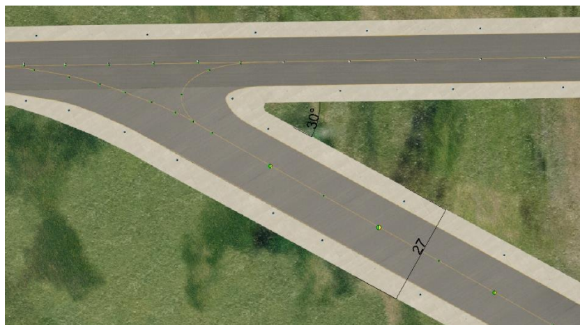
Figure 56: Rapid exit taxiway diagram with beaoning and distances (Source: WED X-Plane developer, Own elaboration)
